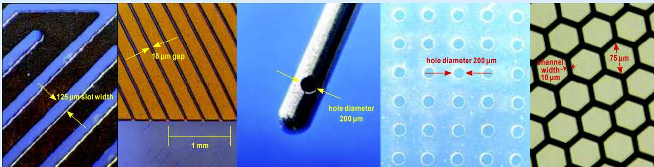
Left to right: 1. 125µm slot in Nitinol 2. 18µm cut in Kapton 3. 200µm hole in SS needle 4. 200µm hole array in polyurethane 5. Hex packed 10µm channels in polymer (Courtesy of Laserlight Technologies)
