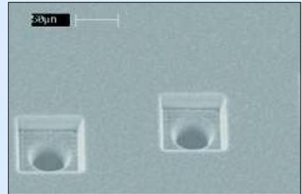
*Ink jet nozzles in orifice plates
